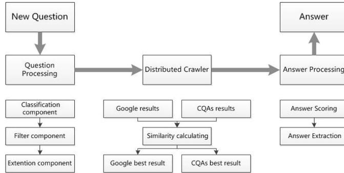
**Fig. 1.** The structure of our QA system
